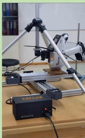
The spectrometer mounted on a tripod during scanning of a panel painting
