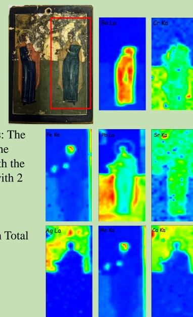
**Elemental distribution maps:** The spectra were acquired by the developed instrumentation with the use of the 3 mm beam spot, with 2 mm step.
