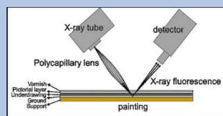
Schematic of the MA-XRF system
