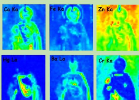
**Elemental distribution maps:** The spectra were acquired by the developed instrumentation with the use of the 3 mm beam spot, with 3 mm step. The analysis was made with PyMCA (Solé, V.A. et al 2007)
