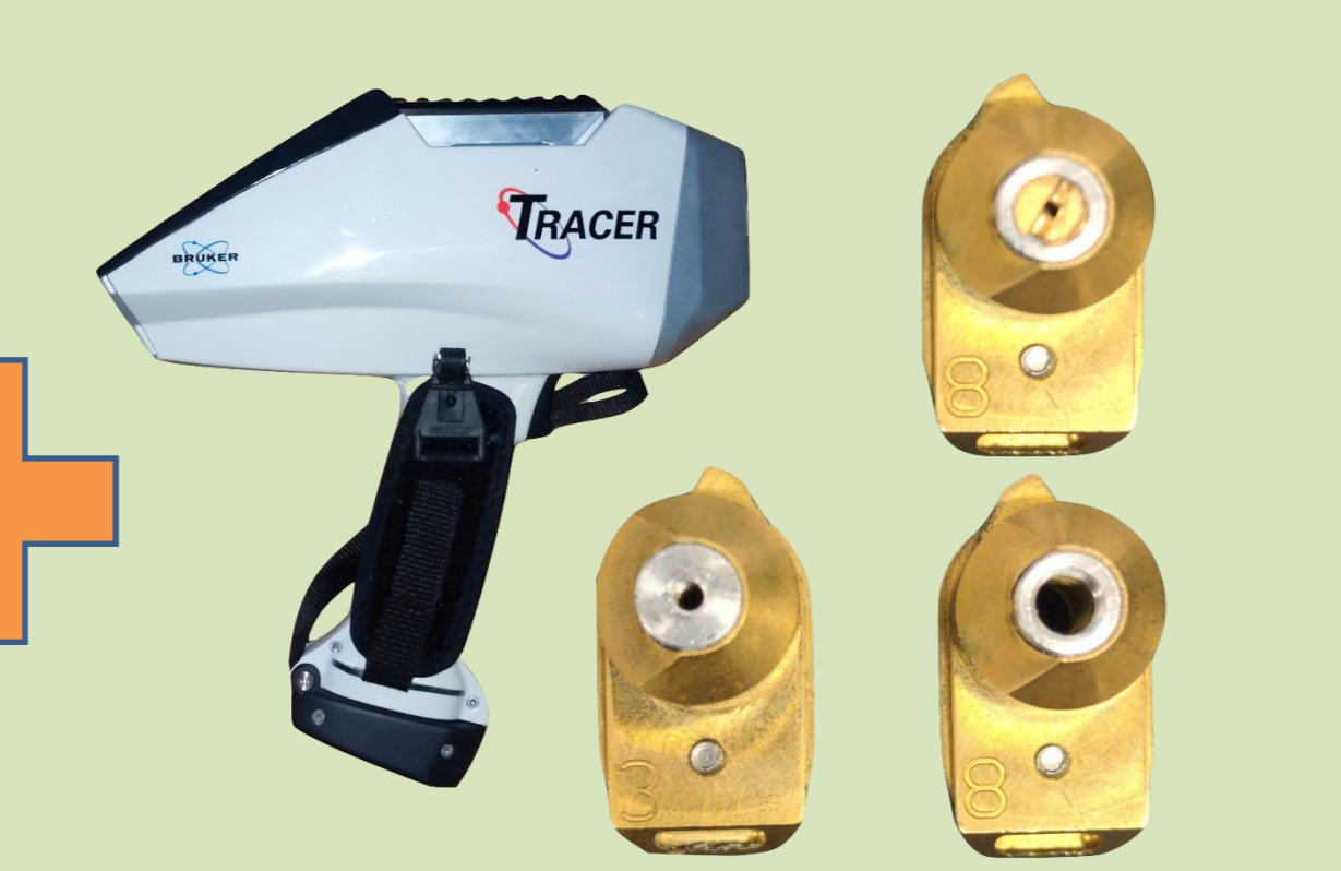
The handled spectrometer (Tracer Si, Bruker) and the original aluminum collimators (3mm and 8mm spot sizes – 2mm and 4.5mm bore size) that accompany the instrument. On top a modified collimator, where a brass thread was drilled to achieve 1 mm beam spot
