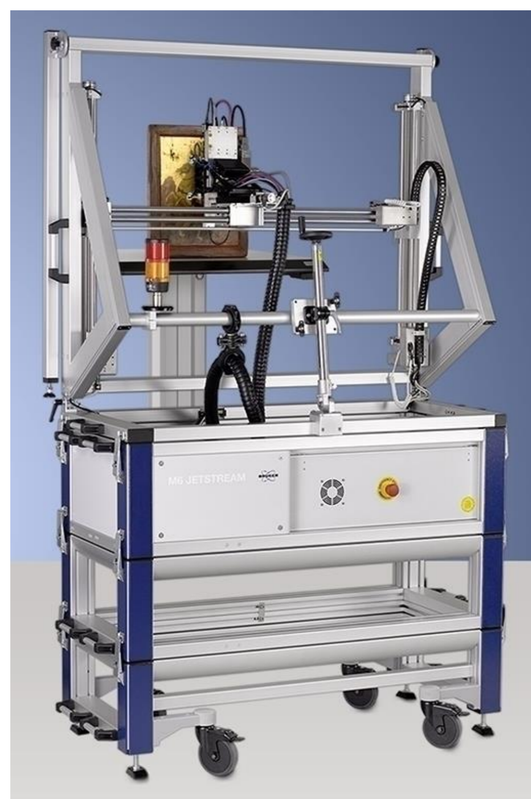
Fig. 2a. MA-XRF scanner. M6 Jetstream (Bruker)
