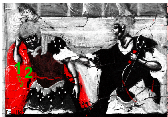
Fig. 8. Left : Overlap of the elemental distribution maps of Pb (white) and Hg (red); the green-highlighted areas 1 & 2 correspond to the areas of the sum spectra shown on the right. Right : sum spectra from areas 1 (red line) and 2 (blue line) shown on the left.
