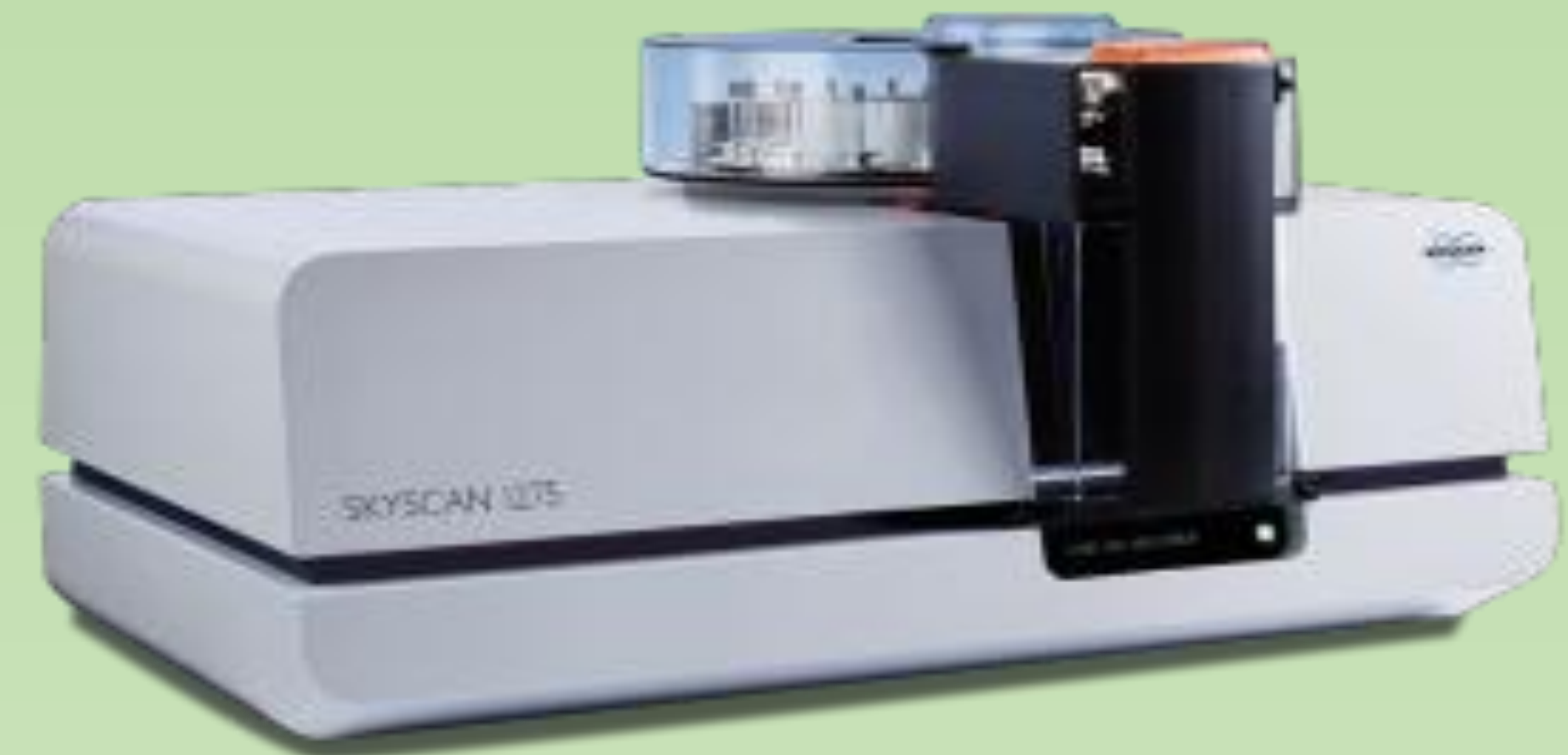
Fig.1: 3D X-Ray microscope (XRM) SKYSCAN 1275, Bruker (Object size: 96mm diameter, 120mm height) [7]
