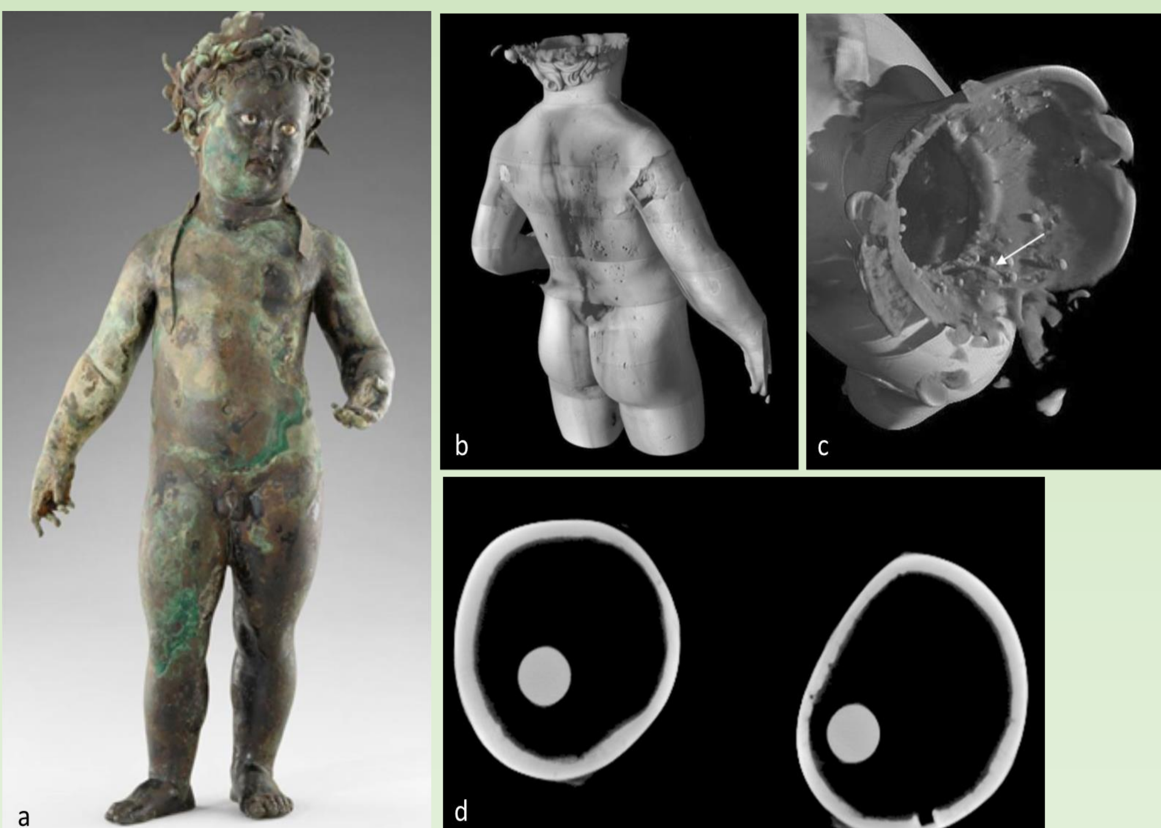
Fig.2: Roman Cupid statue: a) Overall front, b) 3D rendering of the exterior reveals areas of thin bronze in lower back, extensive porosity and repair, c) Interior of head with filled core bubbles. Note neck join (arrow), possibly due to metallurgical work, d) CT section of upper legs showing variable wall thickness and shape. The square feature at lower right is a repaired chaplet hole. Round features are modern pins [5].
